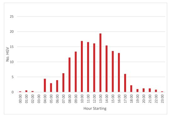
4.3.4 **Figure 11** shows the recorded combined inbound and outbound profile of HGV trips to and from the site.
